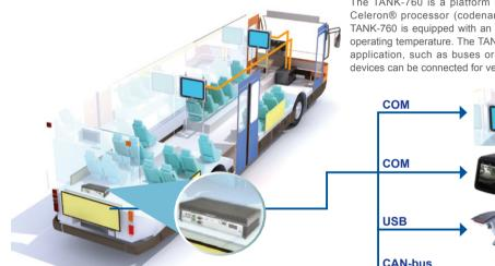
The TANK-760 is a platform based on the 4th generation Intel® Core™ i5 or Celeron® processor (codenamed Haswell) and the Intel® HM86 chipset. The TANK-760 is equipped with an abundant of I/O ports and supports a wide range of operating temperature. The TANK-760 can be used as a control center for in-vehicle application, such as buses or trucks. With dual CAN-bus port, more peripheral devices can be connected for vehicle applications.
