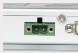
Phoenix terminal using fastening type power connector
